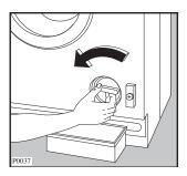
Unscrew and remove the filter.
